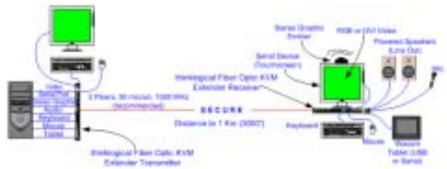
<VIS-1 KVM Extender Connection Diagram>
