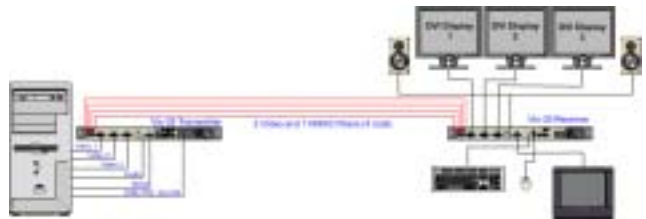
<VIS-35 Triple-head DVI KVM Extender Connection Diagram>
